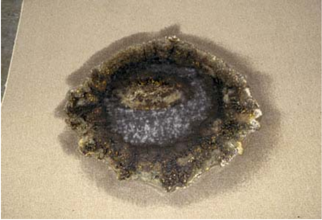
Figure (a) Doughnut burn pattern on carpet, 250 mL gasoline fire, extinguished at approximately 146 s with CO 2
