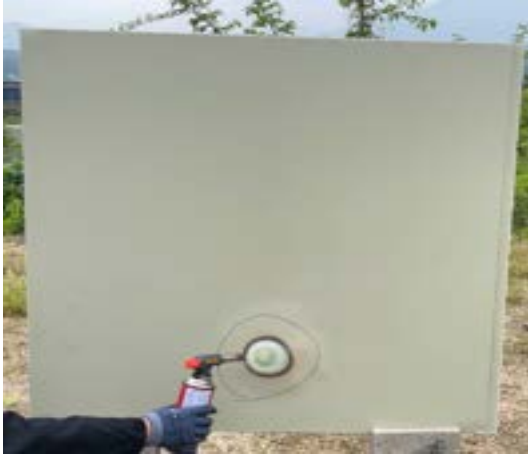
Fig. 9 Sandwich panel Ignition point.
