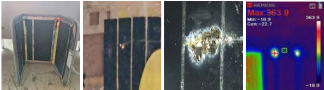
Fig. 25 Heat Film Damage (A사)
