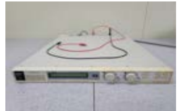
Fig. 12 DC Power Supply
