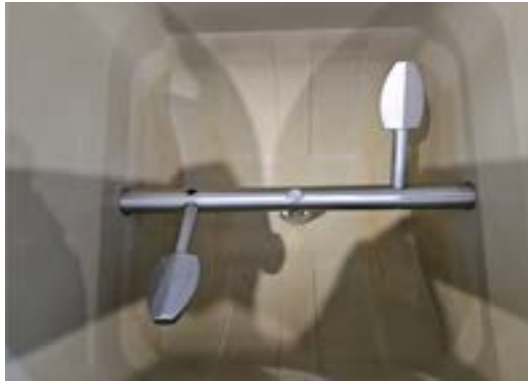
(a) Thermal deformation of bottom plastic structure (Before)
