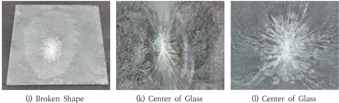
Fig. 17 Combined Heat and Water-Cooling Test on Laminated Glass
