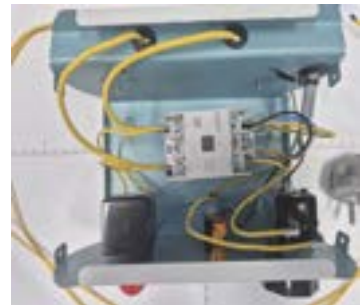
Fig. 3 Internal Structure of a Thermostat
