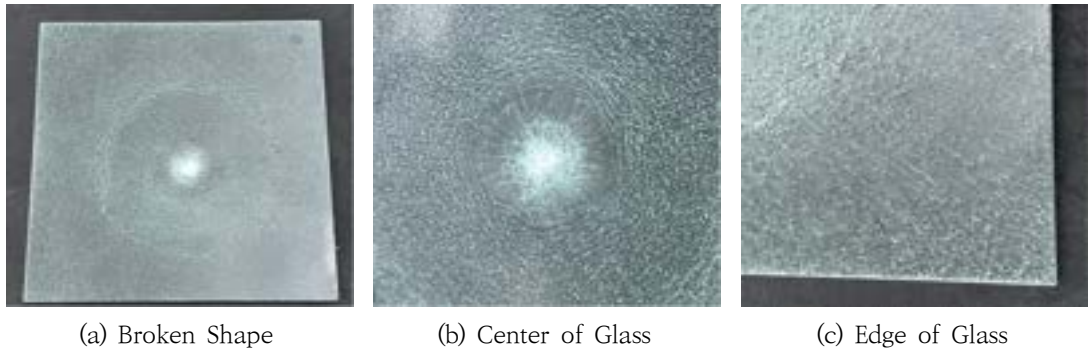
Fig. 14 Impact Test on General Glass Laminated Glass
