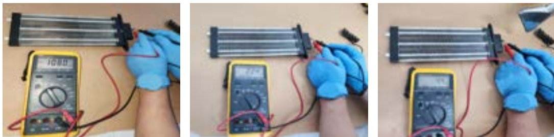
Fig. 14 Measurement of resistance with increasing temperature(108Ω ▶ 22.4Ω ▶ 4.4Ω)
