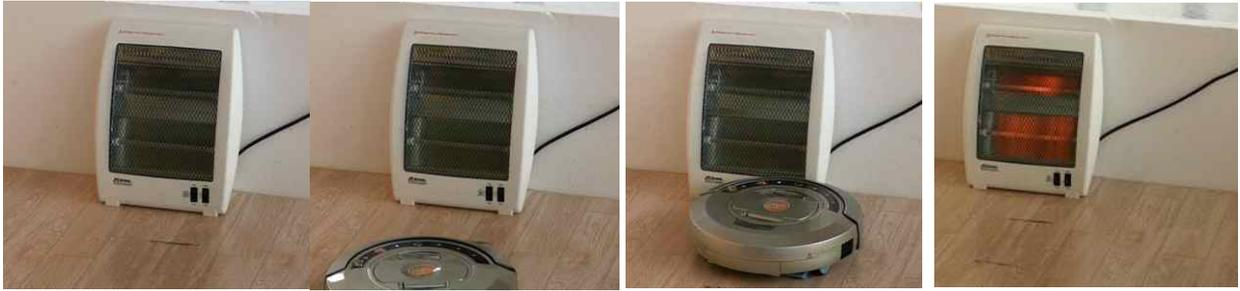
Fig.11 Sequence of unintentional electric stove operation
