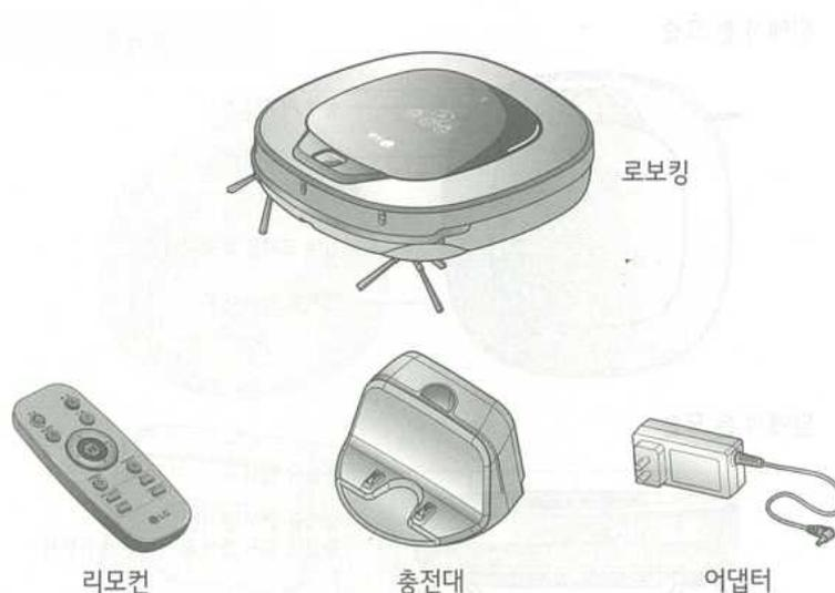
Fig4. Robotcleaner composition
